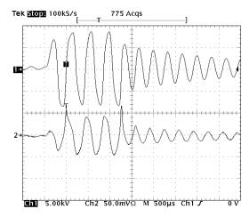
Fig. 18. Voltage(Ch1) and current (Ch2) ) in the secondary side of transformer (applying controls).
