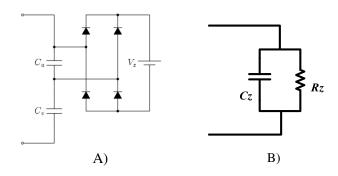
Fig. 1 - Models for ozone generation cell. A) Detailed non-linear model; B) Simplified linear model
