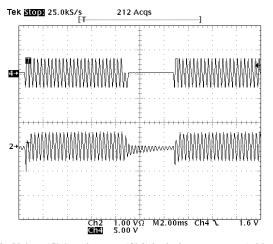
Fig. 13. Voltage(Ch4) and current (Ch2) in the inverter output (with controls acting).
