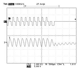
Fig. 14. Detailed view of voltage (Ch4) and current (Ch2) with the application of controls
