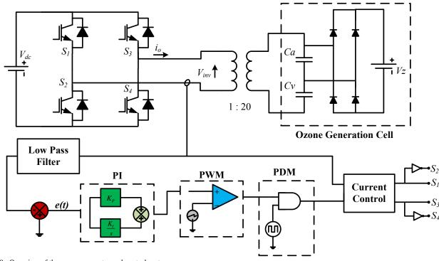
Fig. 9. Overview of the power converter and control system.
