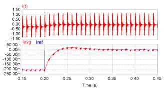
Fig. 8. Response to a step in reference of average current.
