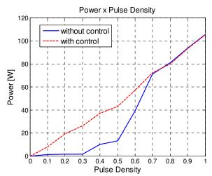
Fig. 15. Relationship between pulse density and inverter output power for controlled and non-controlled version.
