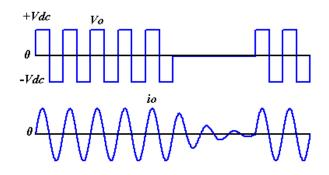
Fig. 4. Standard switching operation in PDM.
