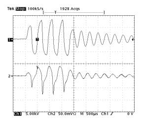
Fig. 17. Voltage(Ch1) and current (Ch2) ) in the secondary side of transformer (without applying controls).
