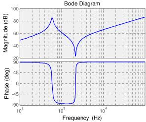
Fig. 10. Bode diagram of the whole transformer plus load.
