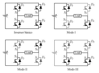
Fig. 3. State of the switches operating in PDM.
