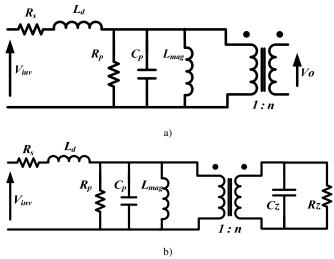
Fig. 2. a) Transformer simplified model; b) Ozone generation cell connected to the transformer
