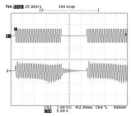
Fig.12. Voltage (Ch4) and current (Ch2) in the inverter output (without the application of control).
