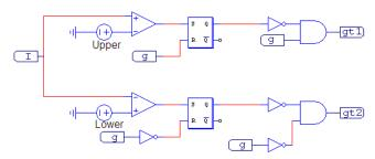
Fig. 6. Current control circuit.
