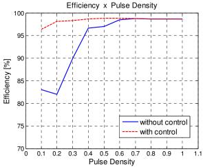
Fig. 16. Relationship between pulse density and inverter efficiency for controlled and non-controlled version.
