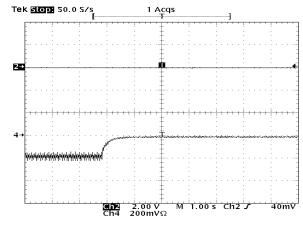
Fig. 11. Response of PI to a step in the reference. Ch2 shows the average output current.
