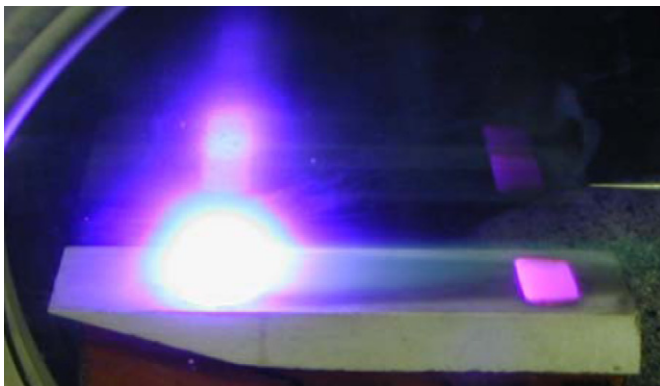
Fig. 13. A DC voltage discharge between two electrodes at freestream conditions of M = 5.15 and p = 0.59 torr. The applied voltage is 880–920 V at a current of 50 mA. The addition of a magnetic field significantly affects the plasma and creates a virtual hypersonic leading edge strake (from [44]).
